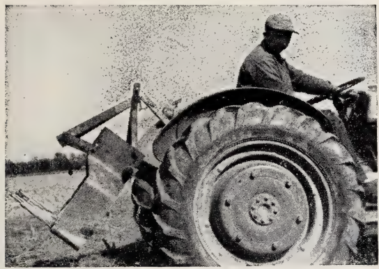
THE CUTTING AND LIFTING BLADE 36 inches wide lifts complete width of row and depth, is hydraulic controlled, assures full and uniform root system under all digging conditions.
